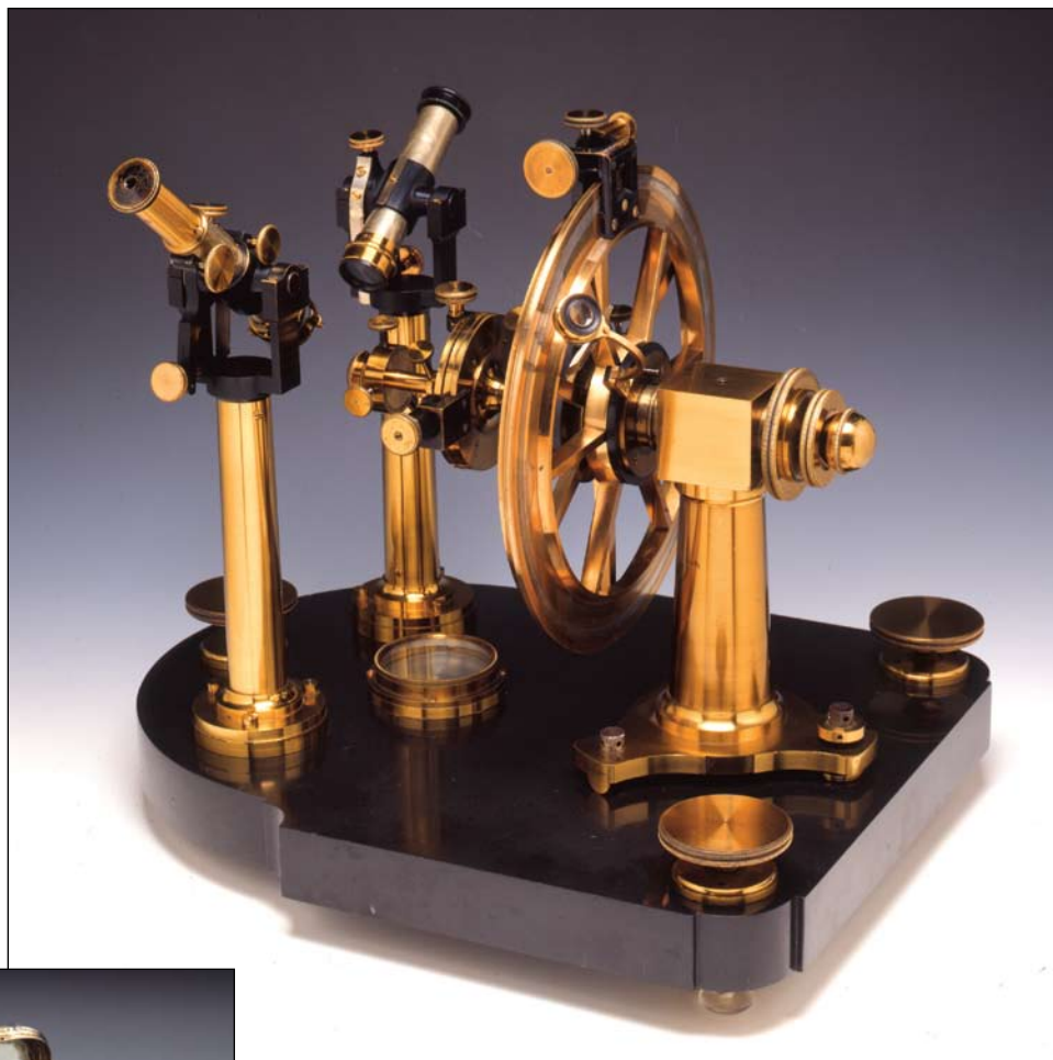
Figure 8. Mitcherlich-type goniometer made by Breithaupt and Sons in Kassel, Germany, dated 1885. Obodda collection; Jeff Scovil photo.
